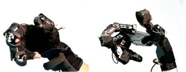
Fig.4. Master Hand vs. 15 DOF Robot Hand Posture
