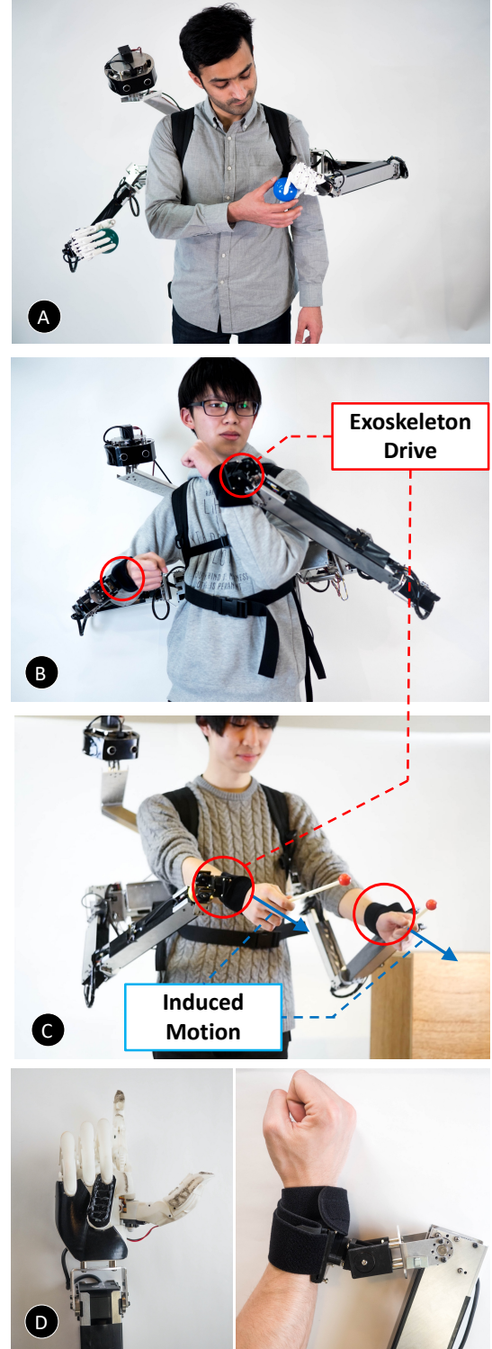
Figure 1: “Fusion” used as a wearable Telexistence system for embodied and physical communication. (A-C) Three levels of communication are realized: (A) Direct Actions , (B) Enforced Postures , and (C) Induced Motion (blue arrows represent the induced motion). (D) End effector can be either a humanoid hand or exoskeleton mount
